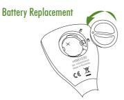
To change the CR2032 Li-ion battery, turn the battery cover located on the back of the meter counterclockwise to unlock. Remove cover and replace the battery with + side facing up.
