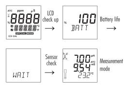
Note: The meter detects the presence and the type of the probe at its input.
