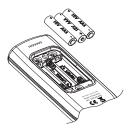
Replace the battery cover making sure that the gasket is in place.
