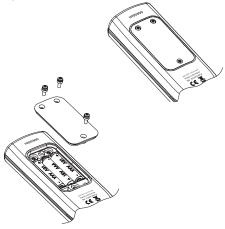
Replace the three 1.5V AAA alkaline batteries located in the battery compartment, observing the indicated polarity.
