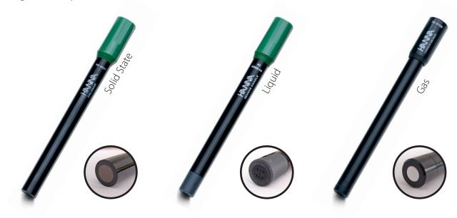
**Solid State Electrodes** are available as both single half-cells or as combination electrodes complete with reference electrode. These electrodes incorporate a solid sensing surface made of compressed silver halides, or solid crystalline material. **HANNN**'s offering includes sensors for the determination of bromide, cadmium, chloride, cupric, cyanide, fluoride, iodide, lead and silver ions. Solid body construction is rugged for long life.
