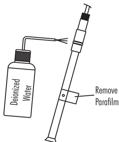
3. Reassemble electrode by gently pushing the inner assembly into the outer body, sliding spring down cable, and screwing cap into place.
