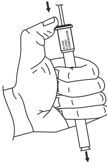
7. Tighten the electrode cap onto the body and fill electrode body until fill solution volume is just below fill hole.
