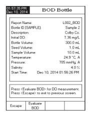
The Current dissolved oxygen measurement of the incubated sample will be made.
