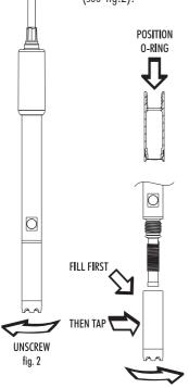
The new membrane cap should be rinsed with electrolyte solution prior to use.
