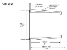
The supplied adjustable brackets allow the controller to slide into the cut-out and hold the unit in place. 95 mm (3.74") is the minimum space required to install the controller with the cables connected.
