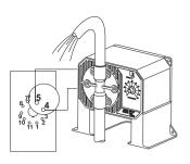
The common terminal (#4) and #3 can also be connected to a device to indicate a "full tank" state.
