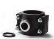
BL120-263 Injector saddle for 63 mm pipe diameter, 1/2" thread
